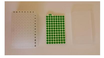
EXAMPLE: 96 well round bottom, 1.2ml wells, sustain steel bead grinding, silicone covers, and box lid
