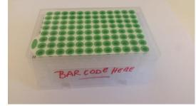
Use deep well, 1.2 ml, round bottom (not conical), round wells that sustain steel bead grinding, 96 well plates.
