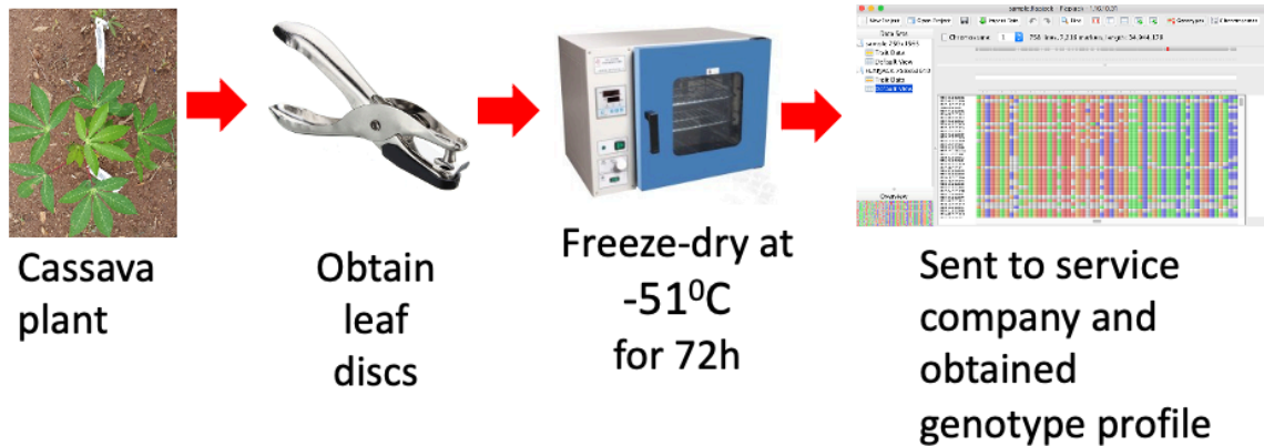
Workflow of tissue sample collection for genotyping at the IITA Cassava Breeding Program
